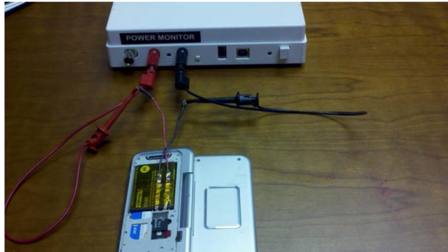
Fig. 4 Power Monitor Setup
